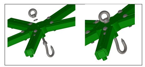
Insert the J-hook through the bottom of Sparrow-B-Gone, place the lock wash onto the top of the J-hook, and screw the top loop onto the top of the J-hook by hand until snug.
